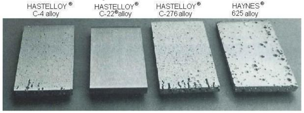
The above image shows the extent of corrosion in the different Hastelloy C series alloys
