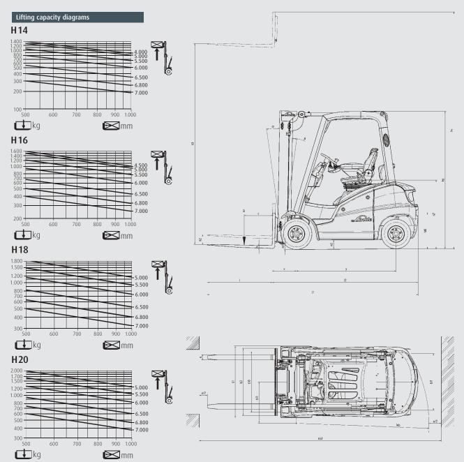
Lifting capacity diagrams are valid for Standard- and Duplexmasts without integrated sideshift with SE-tyres.
