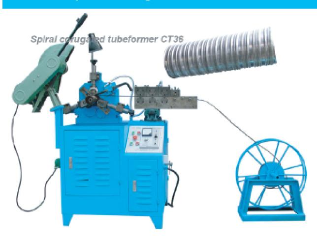
Spiral Corrugated Tubeformer is made for the concrete project, like the bridge building and other kinds of construction. CT78 is widely used in bridgeworks in and out board, which has a compact form and easy to transport. The spiral corrugated pipe machine can be taken to the construction site where the post tension pipe is needed.
