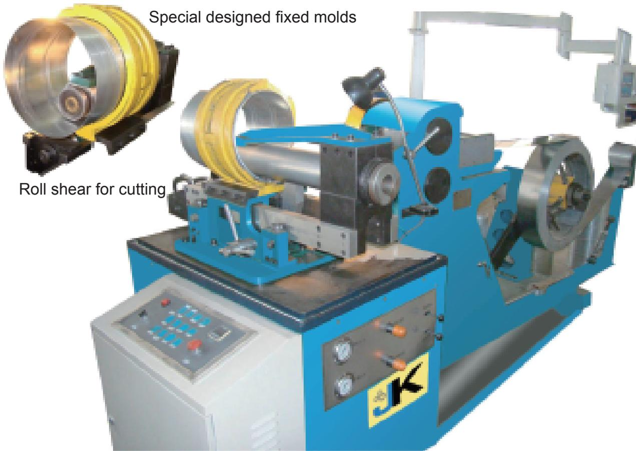
Spiral tubeformer ST150 use the fixed molds, applies the latest flying slitter, which cuts the tubes to length without noise or hot sparks as known from the saws and provides smooth tube ends without deburring.
