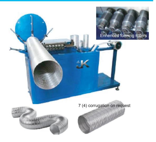
Aluminum tube is widely used in the kitchen, bathroom, air condition venting and HVAC system. The corrugated aluminum tube can easily compressed and strached, and the aluminum corrugat -ed tube can change its shape and keep it.
