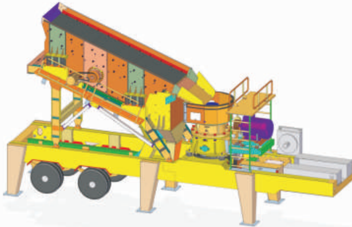
SECONDARY STAGE CRUSHING & SCREENING STATION FITTED WITH CONE CRUSHER
