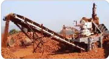
Tertiary Cone Crushers ready to use for iron ore application.
