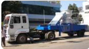
Wheel mounted secondary & tertiary cone crushers.
