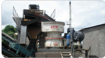
Tertiary Cone Crushers capacities ranging from 40-170 TPH
