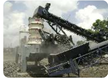
Secondary Cone Crushers capacities ranging from 80-300 TPH
