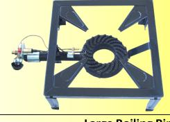
**Large Boiling Ring** 7.5kw (25,500 btu/hr) capacity Boiling Ring Complete with thermocouple and Piezo Ignition Stamped Steel Frame: 400mm x 400mm
