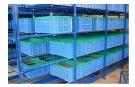
Consist of plastic bins which hold the crushed product and will be placed on the racks. Where every day it has to be subjected to currying.
