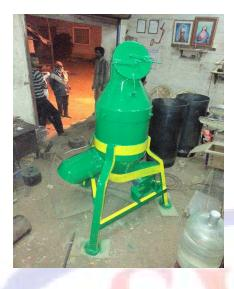
SWS-N Crushing Machine helps to crush all the food waste and vegetable waste and other organic wastes. Blades are made up of <u>SS304</u> Non Corrosive Material. Easy to Operate & Elegant in Design.
